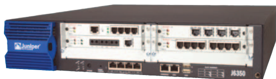
Avaya IG550 Gateway in Juniper J6350 Router
